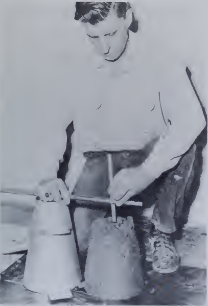
Measuring the slump after subsidence
